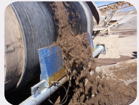
Skalper III belt cleaner in operation at a sand and gravel plant.
