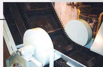
CANTIWHEELS combine the bearings, shafts and wheels in one assembly.
