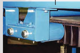
DAMPENING ROLL ASSEMBLIES reduce the pulsations in the belt set up by the belt beaters.
