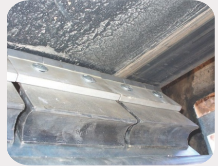
Razor-Back MDX™ with V-tip installed on this conveyor belt at a major copper ore mine.
