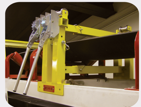
Lifter in action to change out multiple idlers.
