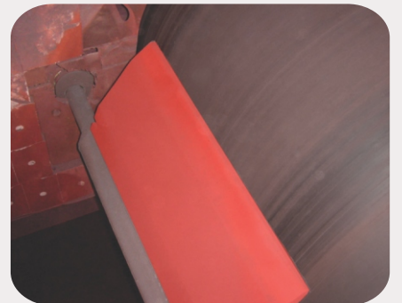
Single piece blade - not segmented - no trapping of materials which may endanger belt life... yet very flexible.
