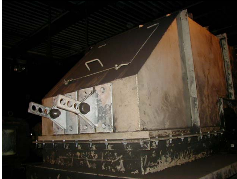
New stainless steel head chute box with the enclosed adjustable ceramic material deflector "Hood".
