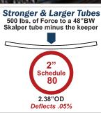
In use with our E-Z Torque® line of tensioner's, our larger mounting tube can eliminate twisting, providing a tension that is distributed evenly across the cleaner blade width along with even wear on the blade, helping to reduce carry-back.
