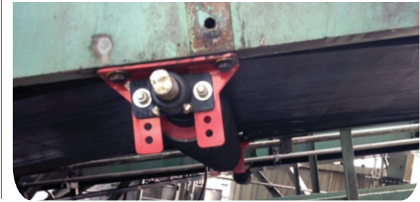
Clamp-Mount™ Skirtboard Sealing System with Tri-seal™ Help eliminate spillage and dust in the conveyor transfer point with clamp-mount.
