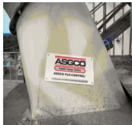
Material is now center loaded onto the screen, increasing capacity and reducing the truck unload times.
