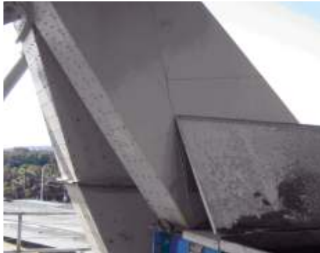
Original chute would build up and plug as well as off center load the screen.
