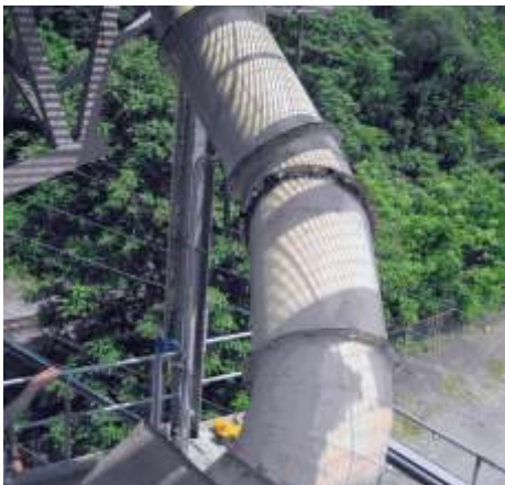
ASGCO Flo-Control curved chute solved plugging and sticking problems without vibrators or UHMW liners
