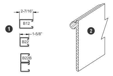
Weld the channel supplied with your system to the existing steel skirt structure at the dimension shown in either illustration A, B, or C. Then lay the sealing compound on the belt with the nub toward the channel. Using a hammer pound the compound into the channel opening. If the section of skirting is less than 20' the E-Z Mount compound can be slid in from one end.
