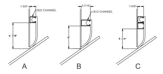
If you were supplied with the B22B type channel, adjustment for wear is accomplished as shown below. Simply move the sealing compound from the top channel to the lower channel when the initial installation is hanging straight down, as shown.
