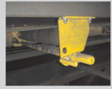
Easy installation and adjustments with beam clamps and chains.
