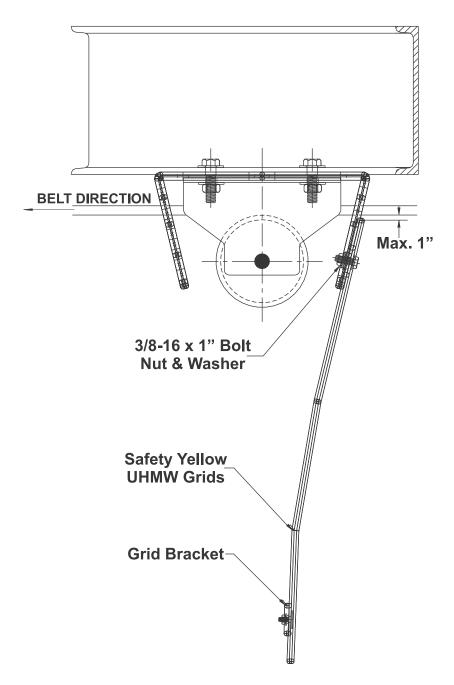
Mount the assembly as shown allowing no more Then 1" between the top of the UHMW grids and the conveyor belt. We recommend the use of a MSHA Approved GO-NO-GO gage to ensure proper adjustment.
