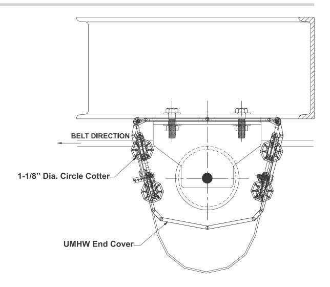
Slide the Safety Yellow UHMW End Covers over the tabs that are on the SAFE-GUARD Mounting Brackets and push down The End Covers should slide down behind the tabs. Next place a Circle Cotter
