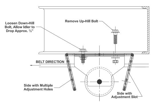
The mounting brackets are slotted on one side so the bracket can slide over top of the idler bracket with the down stream bolt still in place. The up stream bolt should be removed then returned once the SAFE-GUARD mounting bracket is in place. Make sure the four tabs on the mounting bracket are facing away from the conveyor belt.
