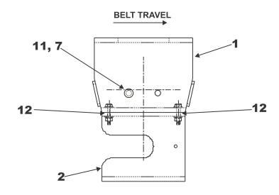
**B.** Attach upper off-side bracket to lower off-side bracket, used 3/4" x 7" pivot bolt and hardware supplied.
