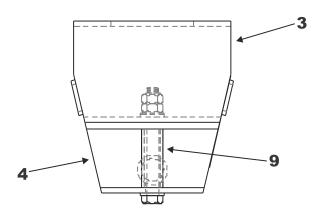
**C.** Attach both on-side and off-side brackets to conveyor steel using  $\frac{1}{2}$ "x 2-1/4" hardware supplied.
