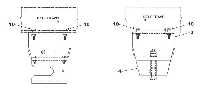
**D.** Attach belt support bar to both upper brackets on the upstream side of the changer using 3/8" x 1" hardware supplied. Belt support bar should be located ½" from the bottom of the belt.
