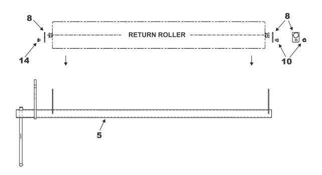
**F.** Slide roller support onto lower off-side bracket pipe.
