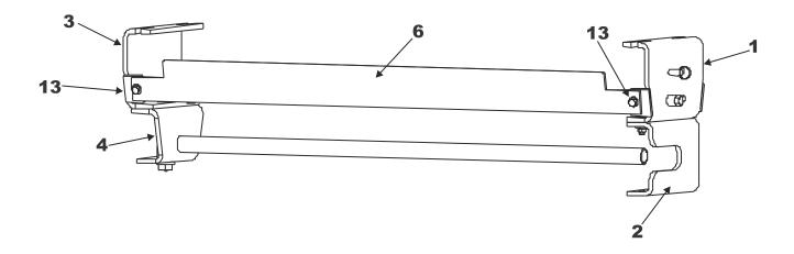
**E.** Install Return Roller onto roller support using roller retainer and 3/8" x ½" long hardware supplied.
