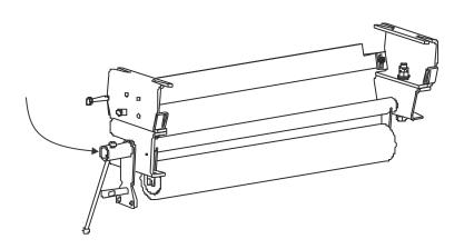
**H.** Rotate roller support upwards so roller comes in contact with belt and handle rests against handle stop. Insert quick release pin through handle and into upper on-side bracket.
