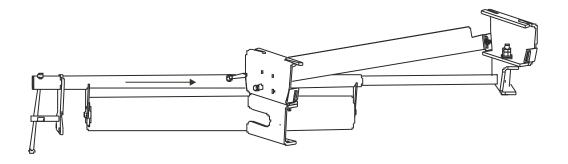
**G.** Swing roller support into lower on-side bracket slot.
