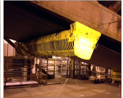
Safe-Guard® Return Idler Guard Installed
