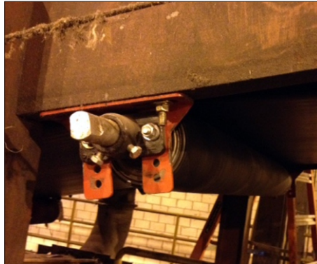
Tru-Trainer® Flat Return Idler Installed
