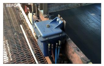
**Before:** This conveyor had a failing hydraulic three return Idler belt training system that wouldn't properly keep the conveyor belt in line.
