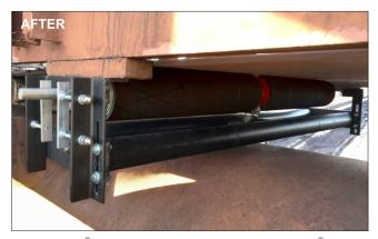
After: ASGCO® engineered low profile Dual Return Tru-Trainer® system with a height of only 11.8", installed to continually recenter the belt.
