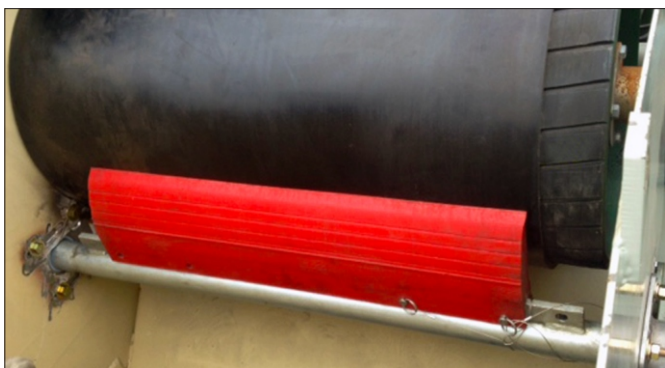
Skalper® with E-Z Torque® installed on the head pulley.
