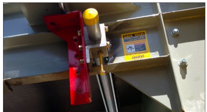
Razor-Back with Bolt-up™ and C-Tip installed after the snub pulley.
