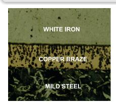
Armorite<sup>®</sup> is an extremely hard (700 Brinell - 63Rc), laminated bimetallic, wear resistant composite. Armorite<sup>®</sup> Typical Bond Zone Product Features:
