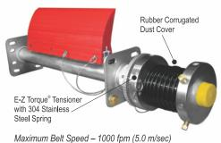
Maximum Belt Speed – 1000 fpm (5.0 m/sec) Pulley Diameter – 16" – 36" (400 – 900mm)
