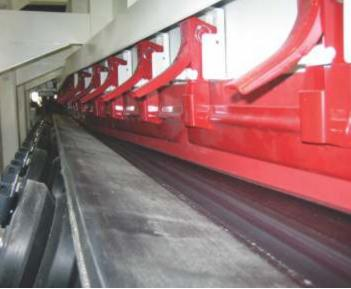
ASGCO® skirt sealing systems and dust control products eliminate spillage, dust and fines at transfer points and provide a highly reliable seal in the load zone.
