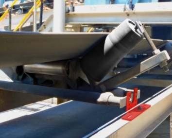
ASGCO®'s line of Tru-Trainer® conveyor belt trackers don't rely on contact with the belt edge in order to guide it. This means that conveyor belt edge damage is avoided.
