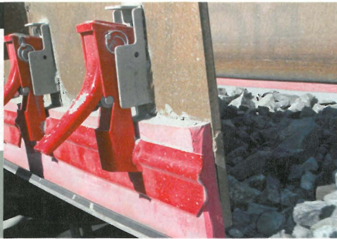
Skirting is a key consideration to prevent material spillage in load zones.
