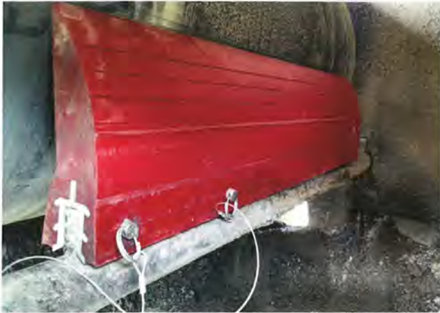
Figure 1. A Skalper with E-Z Torque® tensioner installed on the head pulley for maximum belt cleaning performance.
