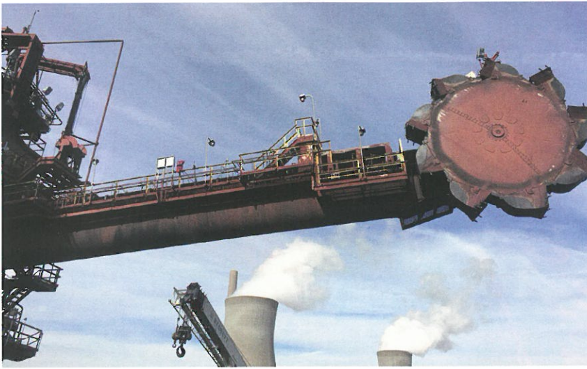
Stacker reclaimer reversing conveyor 60 in. wide steel cable belt.
