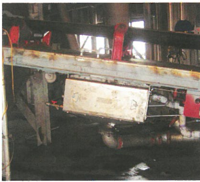
Solution: The ASGCO Wash Box was installed as a secondary conveyor belt cleaner, designed to work on the return side of the conveyor belt.
