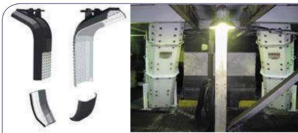
Figure 7. Hood and Spoon Flo-Control chute installation.
