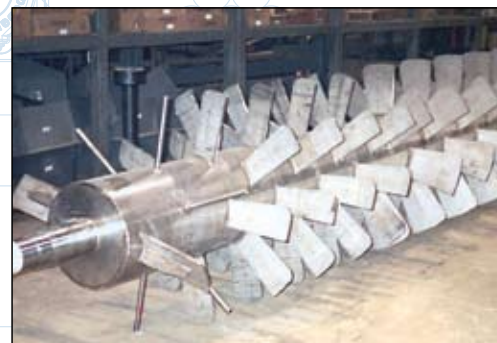
30 ft. long, 48 in. diameter 316SS paddle type screw.
