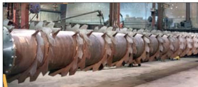
36 ft. long, 38 in. diameter 2205 duplex SS pulp screw.
