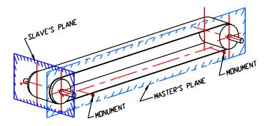
The third planes that are set-up are horizontal, these planes are perpendicular to the master and slave planes and provide a point of reference to measure the deviation from one side to the other of pulley shafts, tripper rails and horizontal conveyor frames.
