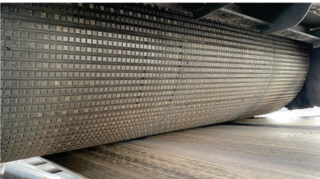
Semi-Ceramic™ Pulley Lagging - Bulk Shipping Terminal Installation
