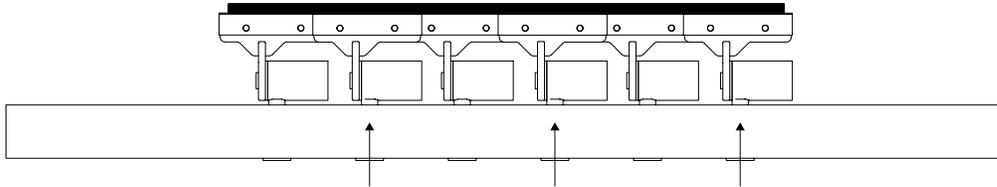
Adjust the rear blade tips so that they are fully contacting the belt surface and tighten the lock nuts.
