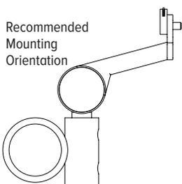
It is important to note, if using optional mounting positions over recommended mounting positions, rotate tube along the tube axis, not end over end. This will ensure the A and B sides of the tube remain in the correct orientation.
