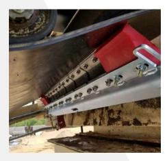
Primary belt cleaners are installed at the 9 o'clock position on the face of the head pulley, referred to as the primary position. It should be mounted below the trajectory flow of the material being discharged from the belt. These are the most common type of belt cleaner.
