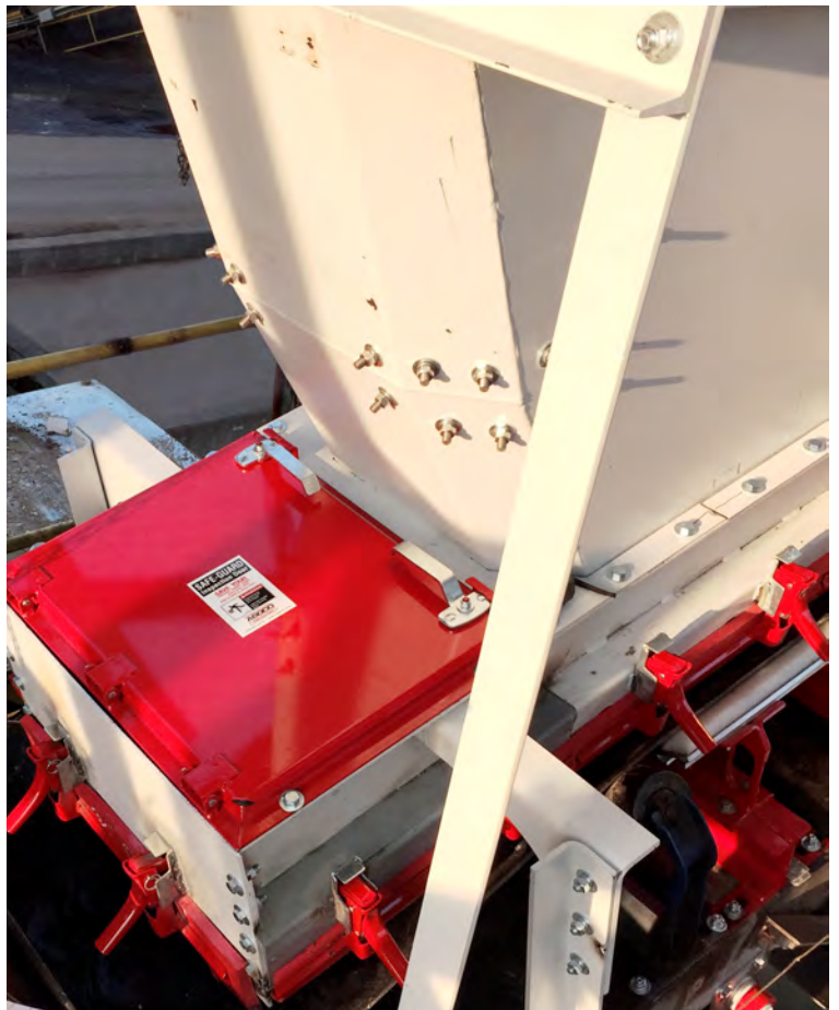
Chute Tail Box
