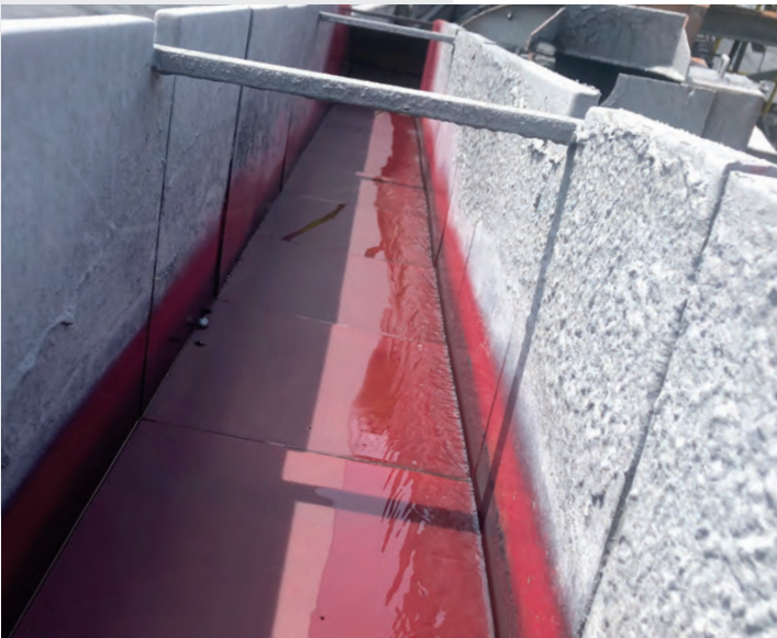
X-Wear™ Urethane Magnetic Liners
