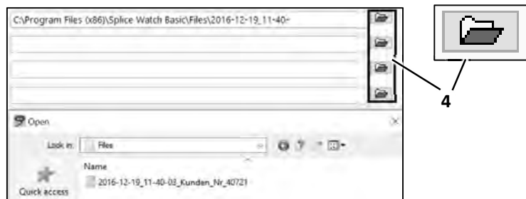
Fig. 25: Selecting the switch box files
